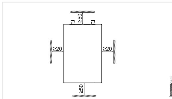
► Maintain the minimum clearances to ensure trouble-free operation of the appliance and facilitate maintenance work.
